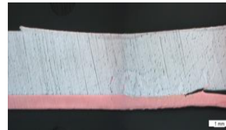
Aluminum sheet and copper sheet lap-welded
